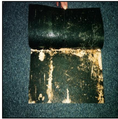
Old Black Cut-Back Asphaltic Based Adhesive
