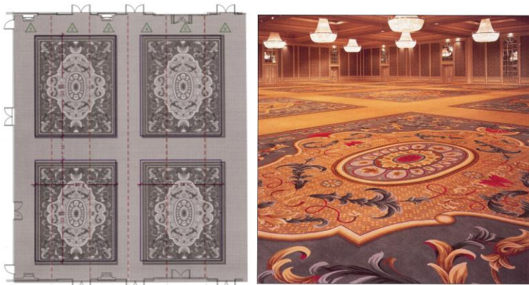
Installation - Seaming Diagram and Completed Installation – Couristan Carpet
