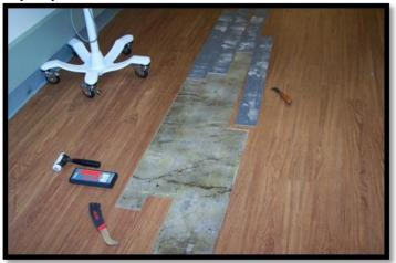
With hard surface products such as sheet vinyl's we can perform tests to determine if the wear layer is as thick as it's supposed to be and whether the product will perform, as well as determine if the product is dimensionally stable or will remain flat.
