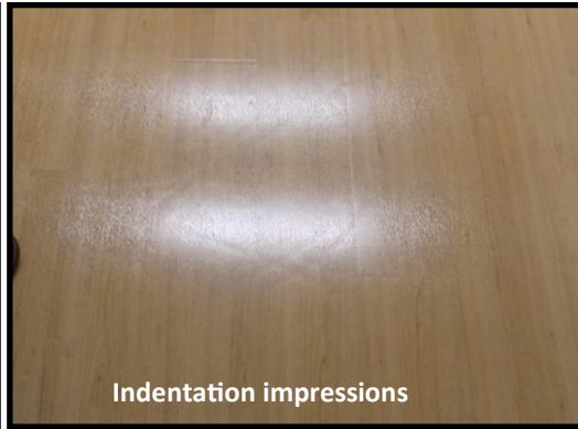
Indentation impressions in adhesive on back of vinyl plank
