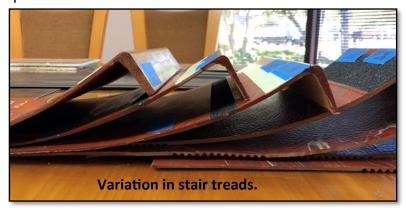
In another case, luxury vinyl plank was installed in a multi-family condo project. The problem was the vinyl shrinking. The shrinking was blamed on installation. Fortunately, we had pictures of the flooring as well as having looked at it physically on two occasions. The manufacturer insisted the problem was installation. The flooring was adhered so tenaciously that it could not be pulled up without heating it and even then it peeled apart. The material continued to shrink.
