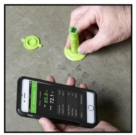
Leapfrogging is never a problem when using single-use RH sensors because they don't get removed and transferred to another test hole.
