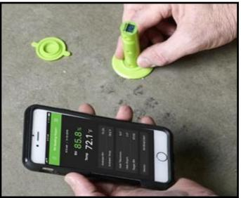
The DataMaster L6 app provides error-free, wireless transfer of your concrete moisture data to your mobile device.
