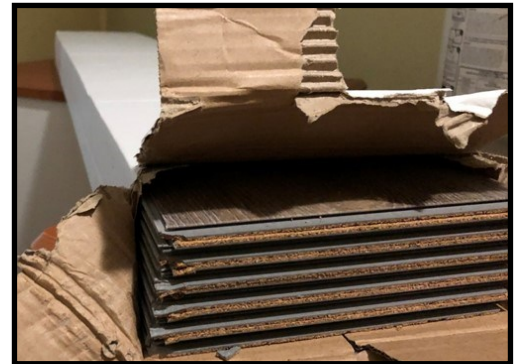
BOX OF ATTIC STOCK OPENED REVEALING DAMAGE TO CORNERS OF FLOORING AND PLAIN WHITE BOX
