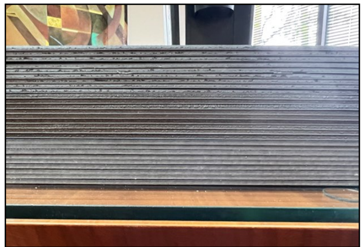
Three Lots of What is Supposed to be the Same Product but Each Lot Has a Different Core
