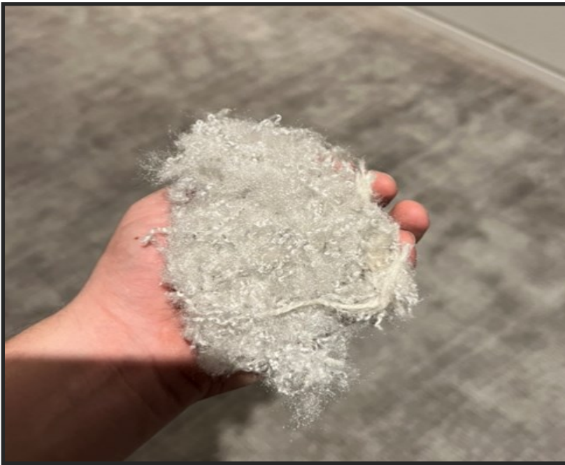
THIS WAS CAUSED BY THE PRESSURE SENSITIVE ADHESIVE PLASTIC CARPET PROTECTOR.
