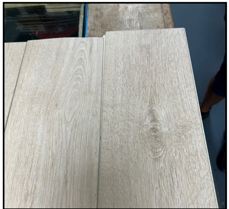
NOTE HOW THE PRODUCT RUNS OUT OF SQUARE FROM TOP TO BOTTOM
